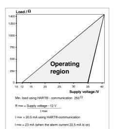
Supply voltage for transmitter without intrinsic safety (not ATEX)
